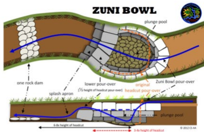
Zuni Bowl Schematic. Figure from Sponholtz, C. and A.C. Anderson (2013)
